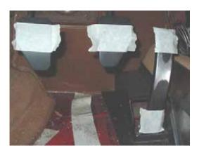
The masking tape will help you see where you have marked the factory clutch/brake pedal sheet metal with the pencil to locate the mounting holes for the aluminum racing pedals.
