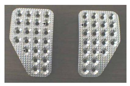
Note: It is our experience that the hole indicated will work for your application, however be sure to confirm that there is ample space on the backside of the factory clutch pedal sheet metal for
